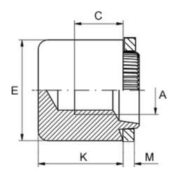
Female thread A = M12Height K = 19.0Min thread length C = 7.0Outer diameter E = 25.0Plate thickness = 2.3 to 2.5
